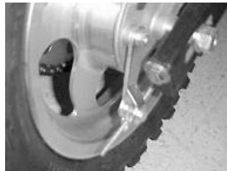
Figure 4, adjust brake lever 'free play'
